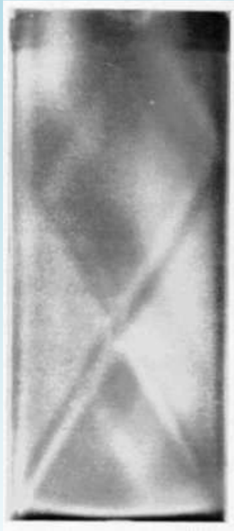
Figure 7: Photograph in the experiment by McEwan. The tank is cylindrical, with its axis aligned to the axis of rotation.
