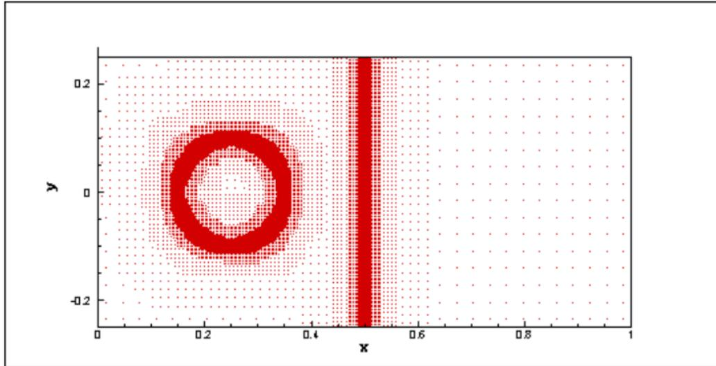
Shock / hot bubble interaction: adapted grid using 9 grid levels.
