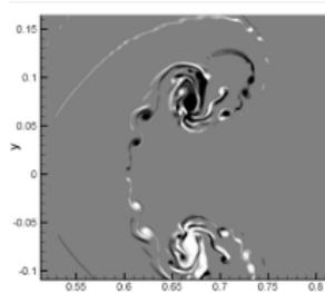
Flame front; diphasic interface; shock/Turbulence interaction; vorticity production by baroclinic effect: need **High-order schemes** + **mesh refinement**.
