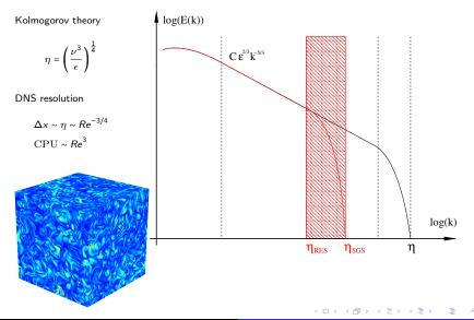
HOM for industrial turbulence Validation Towards real-life applications Cor DNS Taylor-Green Homogeneous isotropic turbulence LES of Homogeneous
