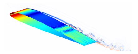
Large Eddy Simulation : solve for low-pass filtered solution  $\tilde{\mathbf{v}}$
