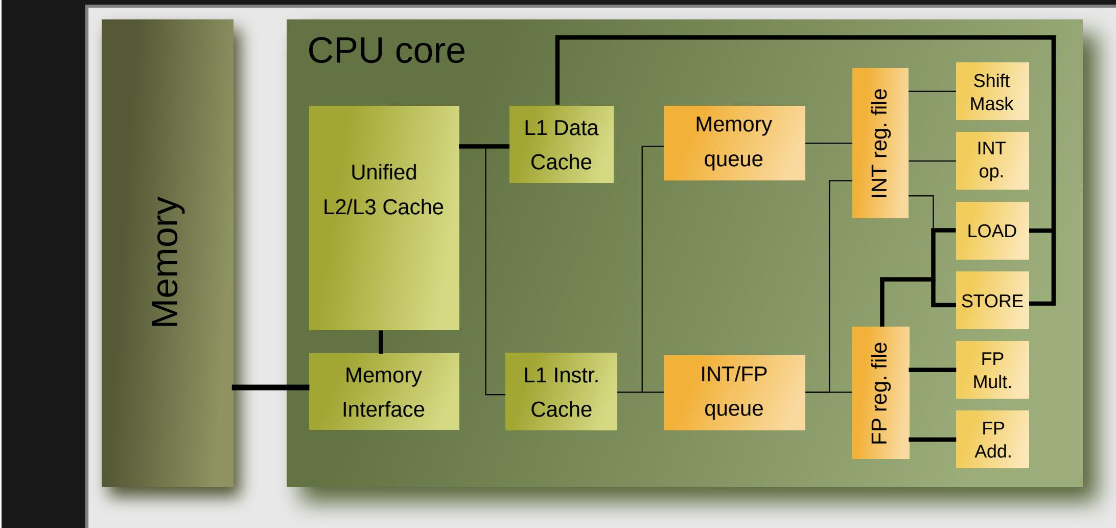
Most of the control unit, e.g. instruction fetch/decode, branch prediction,... not shown
