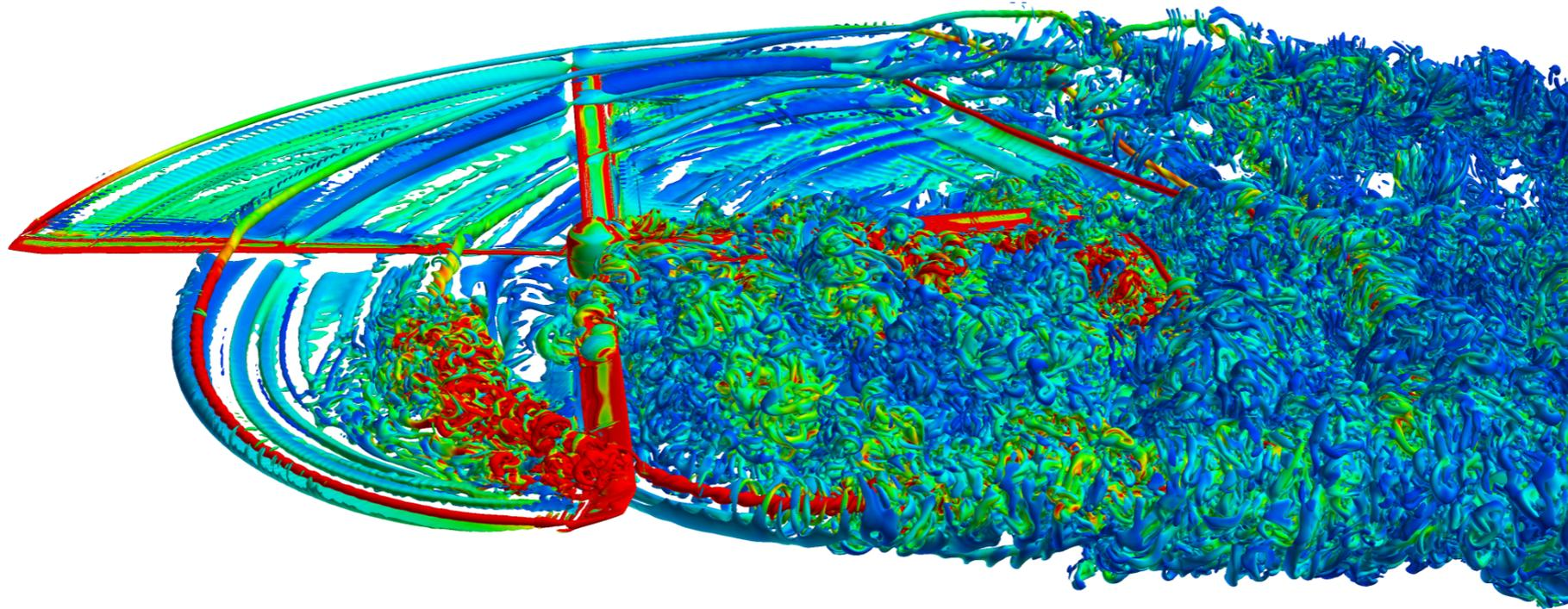
Simulation of dynamic stall for a Blackhawk helicopter rotor in forward flight. (credit: NASA ARC).
