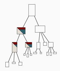
Typically two sources of parallelism are exploited in the multifrontal method
