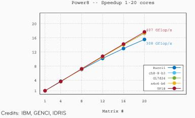
On a 2 x Power8 machine 88% of parallel efficiency on 20 cores
