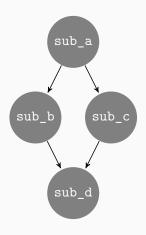
sub\_b and sub\_c can be executed in parallel. If sub\_a is executed on CPU and sub\_b on GPU, x will be automatically transferred.
