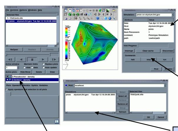
The Simulation's window shows meta-data about the running code
